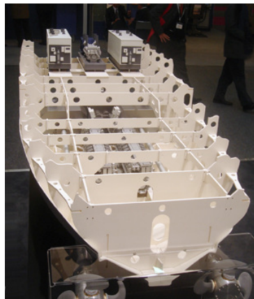
A seven-foot model of MTU's combined diesel and gas turbine (CODAG) for military vessels demonstrates the integration of diesel engines and gas turbine for unrivaled speed and flexibility.
