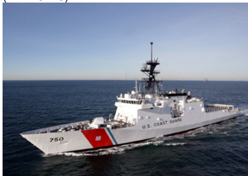
The Legend Class National Security Cutter USCGC Bertholf features MTU's CODAG-propulsion system.
