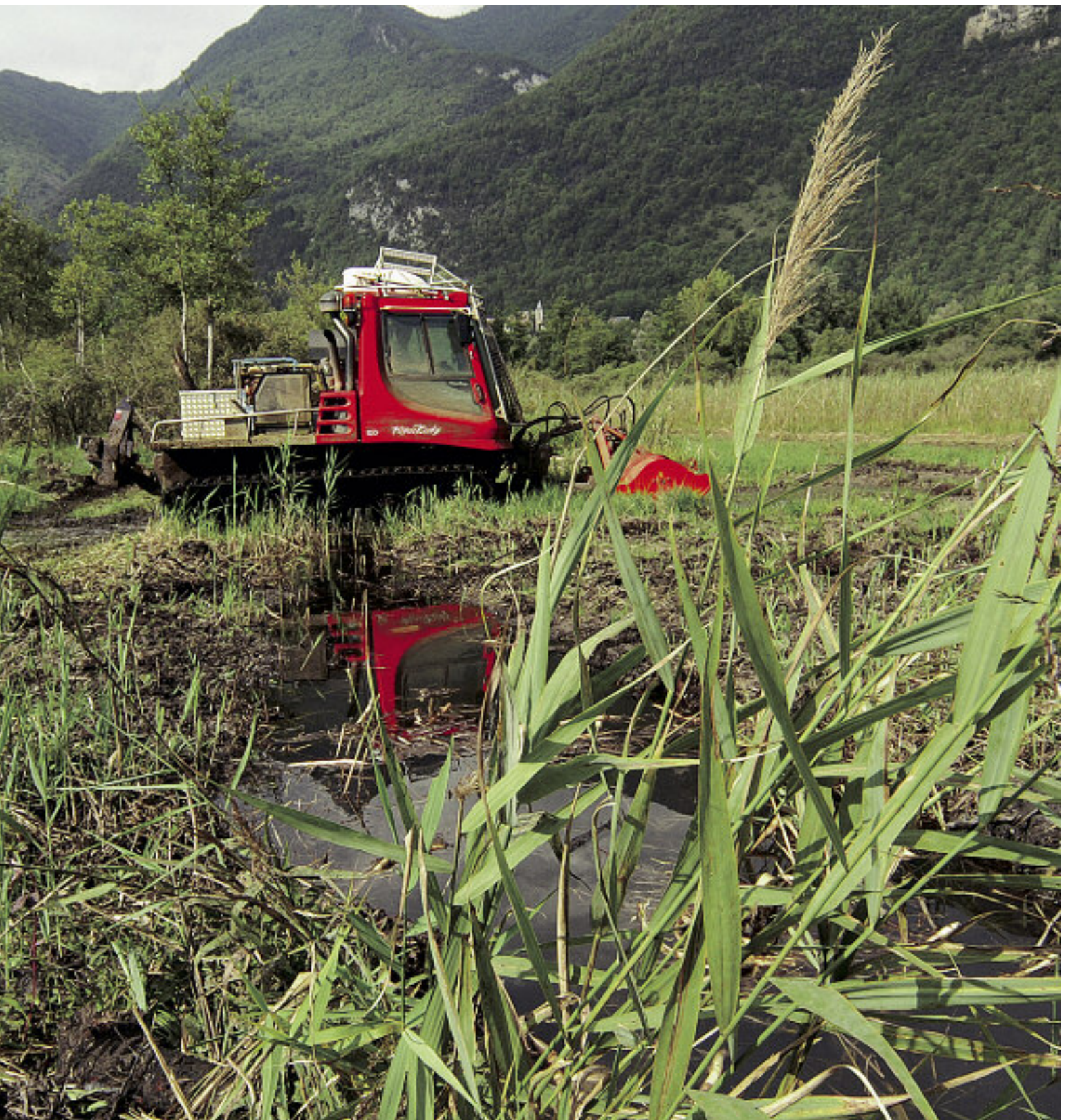
Because of its low surface pressure characteristics, the Pistenbully doesn't sink in even on marshy ground.
