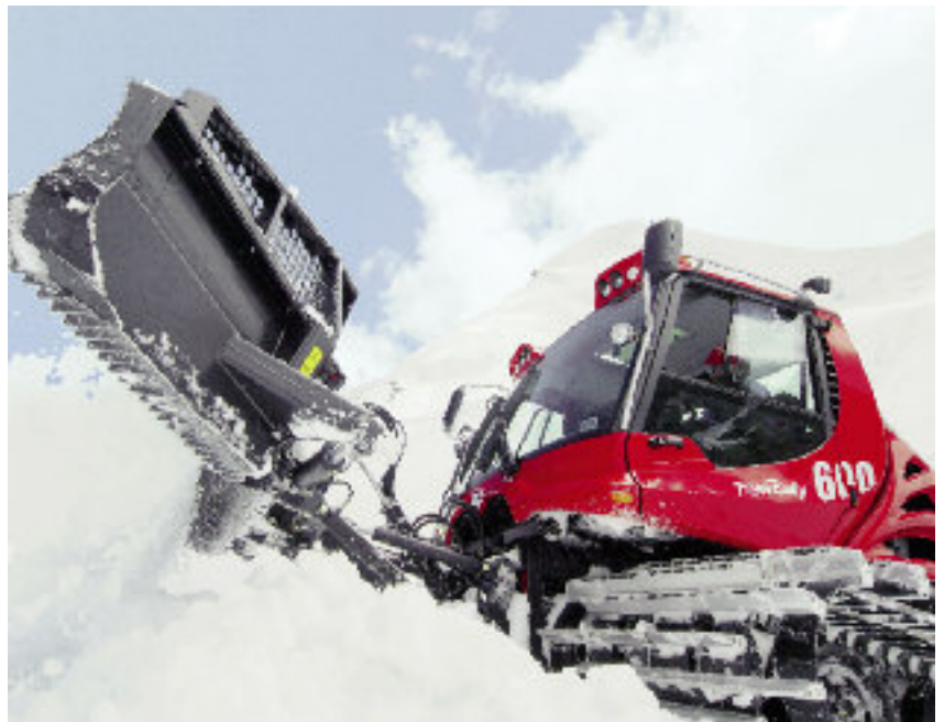
With its special attachment kinematics, the Pistenbully 600 Park is extremely maneuverable. The front and rear attachments can be operated simultaneously.
