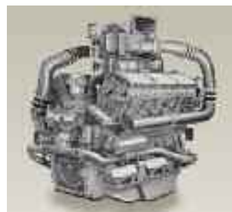
The MD engine (MD stands for Maybach diesel) is Maybach's first modular engine and far ahead of its time. Along with its precombustion chambers, its pioneering design features include the fuel injection system developed together with L'Orange, in which pump and injector are combined in a single unit. That enables the high-pressure fuel lines previously required to be dispensed with and short injection periods to be achieved at moderate pump pressures.
