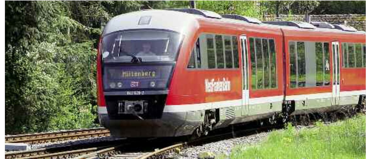
Up to now the VT 642 railcar has been driven by a conventional MTU PowerPack. Now it is to be fitted with a hybrid system.
