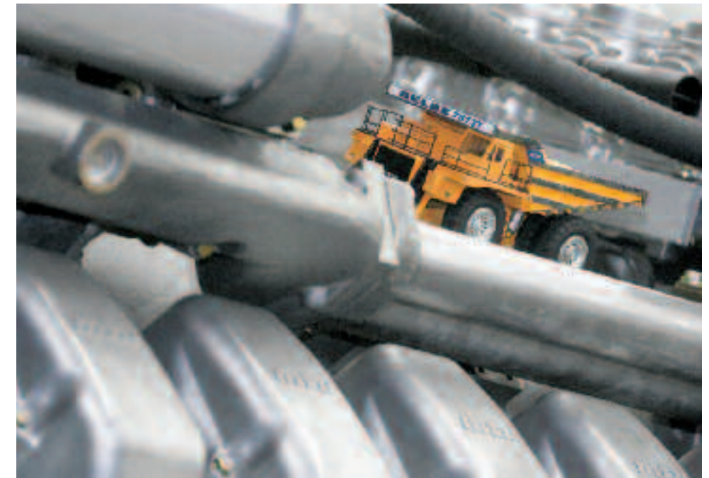
MTU Series 4000 engines power the biggest dump trucks on Earth. They have water-cooled exhaust pipes to minimize fire risks.
