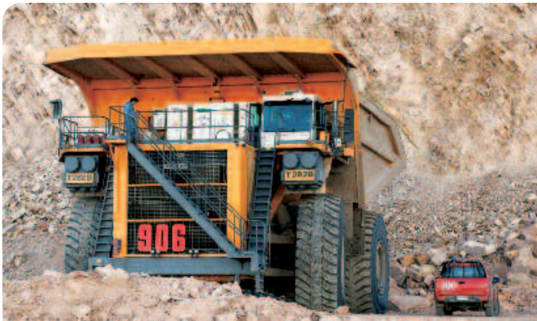
They are the true giants of mining. The dump trucks stand nine meters high and weigh 600 tonnes. Next to them, ordinary cars look like toys.
