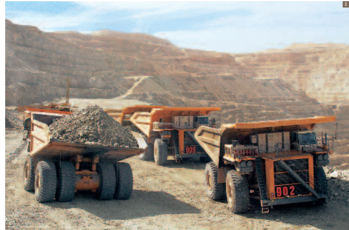
1 It takes just under an hour for a dump truck to transport its valuable cargo from the bottom of the pit up the terraced slopes to the top of the mine. 2 There are 125 dumpers in use in Chuquicamata, each of them capable of carrying up to 400 tonnes of copper ore.
