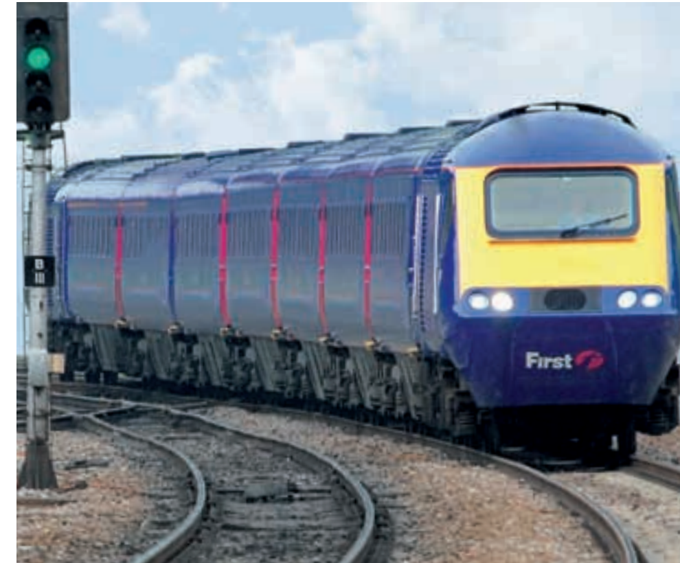
One of the biggest repowering projects completed by MTU involved refitting British HST power cars with Type 16V 4000 engines.
