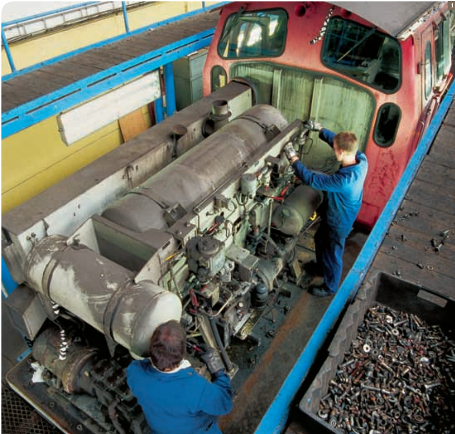
1 Repowering a V290 locomotive: at the Deutsche Bahn repair depot in Cottbus, 400 of these locomotives have been refitted with MTU 8V 4000 engines. 2 Re-equipped with Series 396 engines, Russian DR1A trains can continue to operate economically. 3 The Alstom locomotives used by the Thailand national railways are being converted to Series 4000 engines because, apart from anything else, they use 28 percent less diesel fuel.
