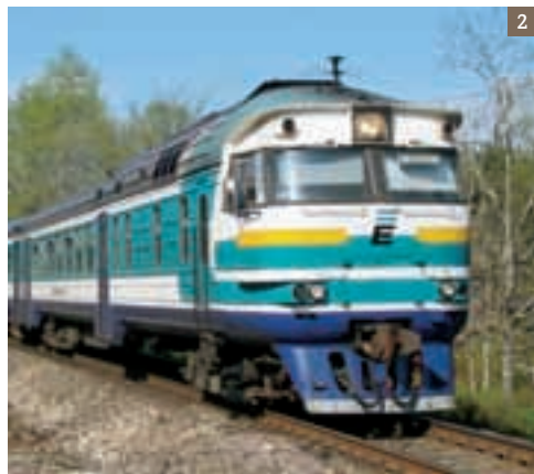
1 Repowering a V290 locomotive: at the Deutsche Bahn repair depot in Cottbus, 400 of these locomotives have been refitted with MTU 8V 4000 engines. 2 Re-equipped with Series 396 engines, Russian DR1A trains can continue to operate economically. 3 The Alstom locomotives used by the Thailand national railways are being converted to Series 4000 engines because, apart from anything else, they use 28 percent less diesel fuel.
