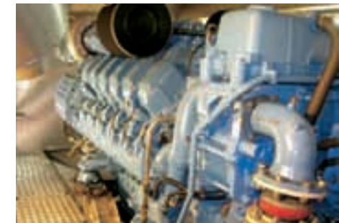
For six years, an MTU Series 4000 diesel was “the best engine in the fleet” of the shipping company Tide Sjö. Now it is being reconditioned for new assignments at the MTU remanufacturing center.
