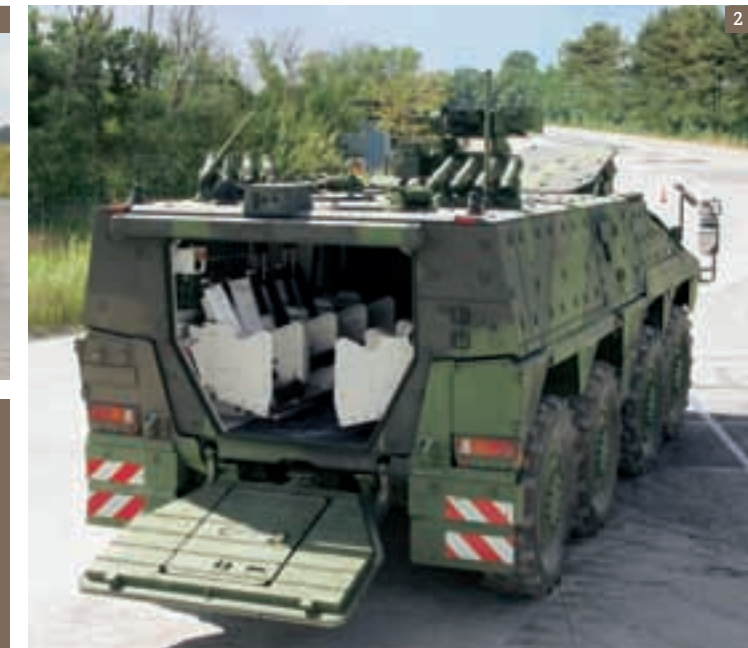
A major advantage is its versatility. The Boxer comprises a base vehicle that is virtually identical for all variations and an interchangeable mission module. Thus the armored personnel carrier (photos 1 and 2) can be converted into a field ambulance (photo 3) in the space of an hour.
