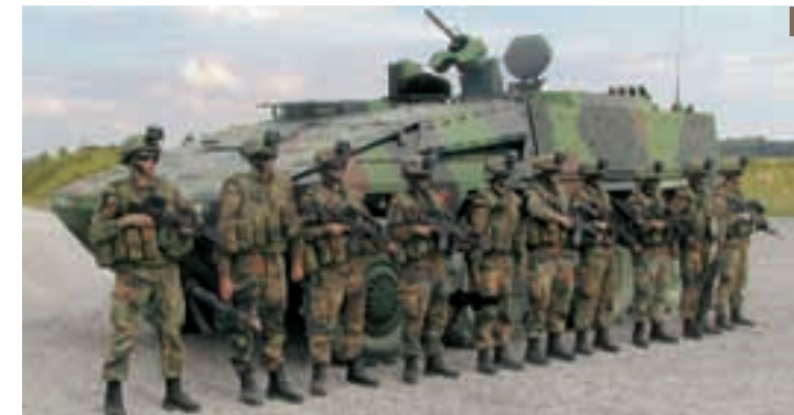
A major advantage is its versatility. The Boxer comprises a base vehicle that is virtually identical for all variations and an interchangeable mission module. Thus the armored personnel carrier (photos 1 and 2) can be converted into a field ambulance (photo 3) in the space of an hour.
