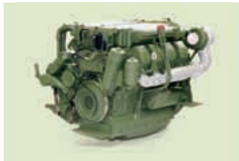
The Boxer is powered by a 530-kilowatt MTU Series 199 engine. It is based on a Mercedes-Benz truck engine. That basic design has been modified by MTU to make it suitable for military applications. The adaptations include improved power output compared with the commercial-vehicle engine and dry-sump lubrication to cope with the extreme inclinations at which it is required to operate.
