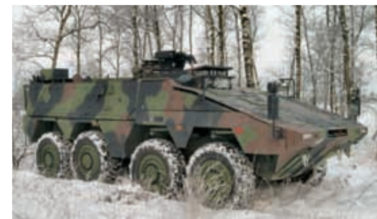
Due to its maximum torque of 2,700 newton-meters, the MRAV has ample power to accelerate quickly to high speeds even on rough ground.
